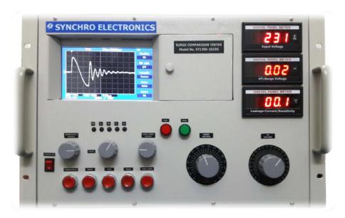
**Synchro Electronics Surge Comparison Tester** not only tests the ground insulation, but it also tests turn-to-turn, coil-to-coil, layer to layer, and phase-to-phase insulation more efficiently. In fact the surge test can detect the fault, even if a single turn is shorted. It can also find out the problems such as reverse or wrong internal connections, wrong turn counts and open coils.
